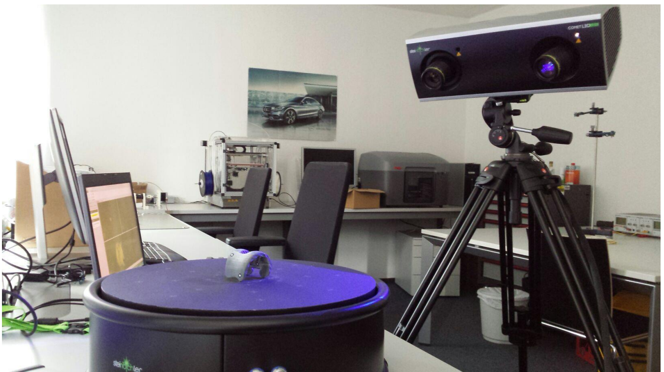
COMET L3D scanning a knee prosthesis
